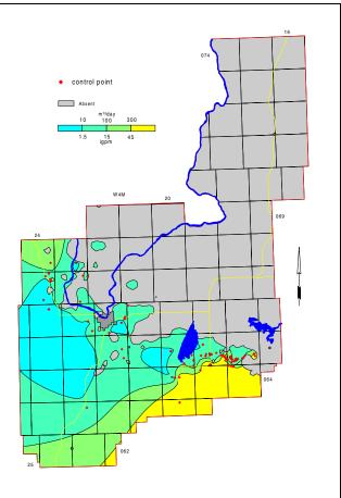
Figure 20. Apparent Yield for Water Wells Completed through Brosseau Member
