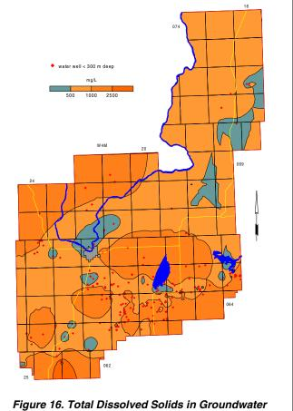
Figure 16. Total Dissolved Solids in Groundwater from Upper Bedrock Aquifer(s)
