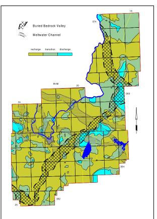
Figure 23. Recharge/Discharge Areas between Surficial Deposits and Upper Bedrock Aquifer(s)
