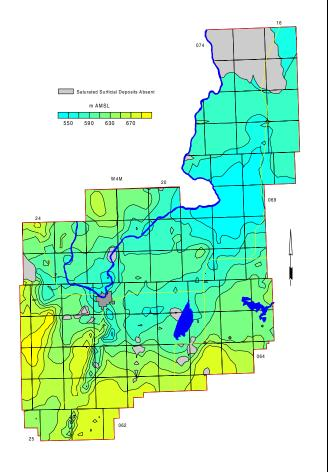
Figure 22. Non-Pumping Water-Level Surface in Surficial Deposits
