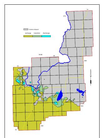
Figure 24. Recharge/Discharge Areas between Surficial Deposits and Victoria Aquifer
