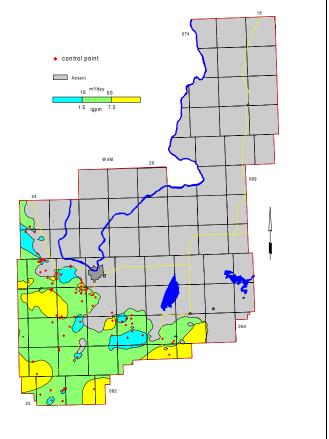
Figure 18. Apparent Yield for Water Wells Completed through Ribstone Creek Aquifer
