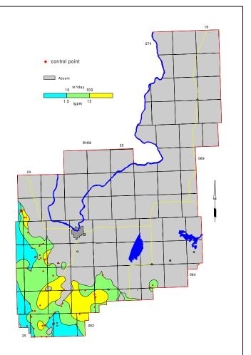
Figure 17. Apparent Yield for Water Wells Completed through Birch Lake Aquifer
