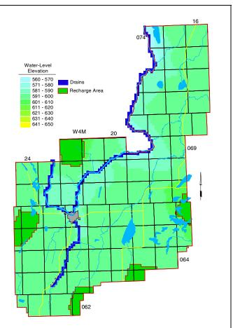
Figure 25. Modelled Non-Pumping Water-Level Surface in Surficial Deposits
