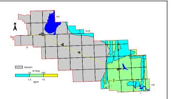
Figure 22. Apparent Yield for Water Wells Completed through marine Foremost Aquifer
