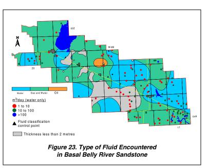
information to allow for the calculation of an apparent long-term yield. The projected long-term yield values vary from less than 5 m<sup>3</sup>/day to a maximum of 16.6 m<sup>3</sup>/day, with the mean being 8.7 m<sup>3</sup>/day and the median 7.7 m<sup>3</sup>/day.
