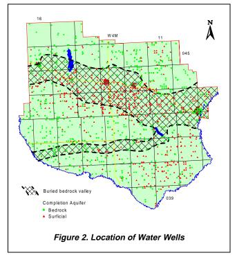
it can be seen that water wells completed in bedrock aquifers occur mainly outside the areas where surficial water wells are completed.
