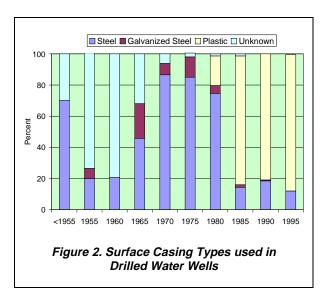
with plastic casing has increased and in the mid-1990s, plastic casing was used in 88% of the water wells drilled in the County.
