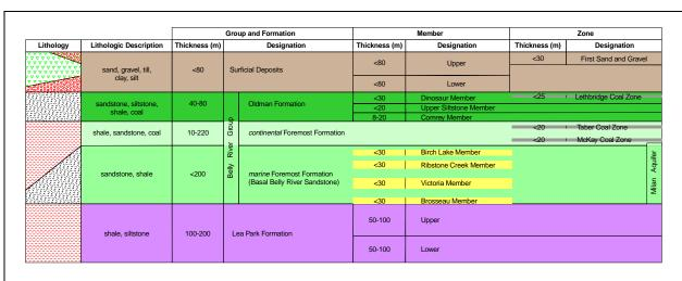
Figure 6. Geologic Column
