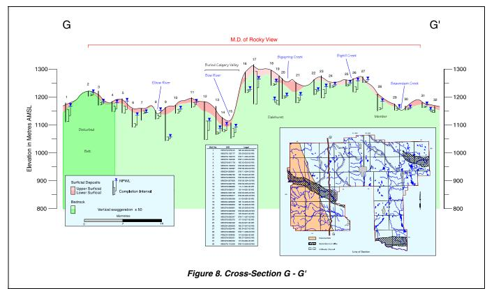
The main aquifers in the surficial materials are sand and gravel deposits. In order for a sand and gravel deposit to be an aquifer, it must be saturated; if not saturated, a sand and gravel deposit is not an aquifer. The top of the surficial aquifers has been determined from the non-pumping water level in water wells that are less than 20 metres deep. The base of the surficial deposits is the bedrock surface.
