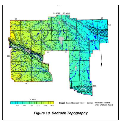
metres. Sand and gravel deposits can be expected in association with this bedrock low, with the sand and gravel deposits expected to be mainly less than 15 metres thick.
