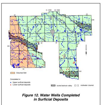
Water wells completed in the upper surficial deposits occur mainly near or within the Disturbed Belt area and in the southwestern part of the M.D. Water wells completed in the lower surficial deposits occur mainly in the vicinity of streams and linear bedrock lows (Figure 12).
