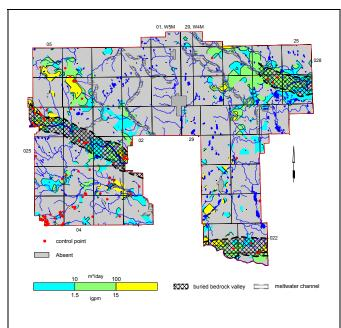
Figure 13. Apparent Yield for Water Wells Completed in Sand and Gravel Aquifer(s)
