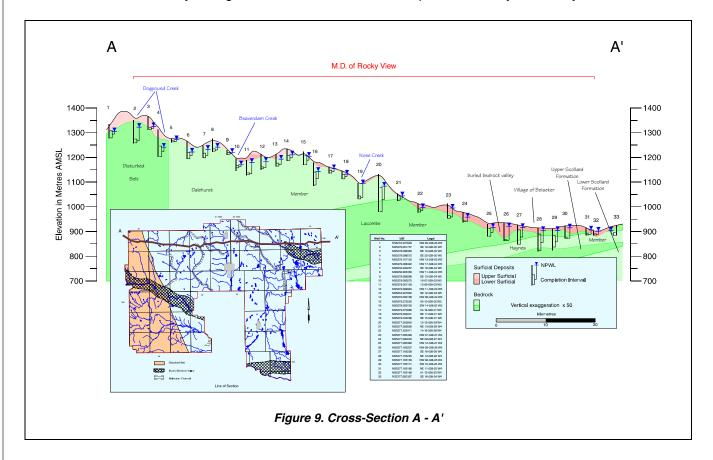
In the M.D., the Base of Groundwater Protection extends below the Upper Scollard Formation. A map showing the depth to the Base of Groundwater Protection is given on page 7 of this report, in Appendix A, and on the CD-ROM.
