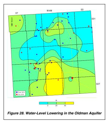
pre-1975 water-level elevations. This water-level decline may be a result of limited recharge to the bedrock aquifers.
