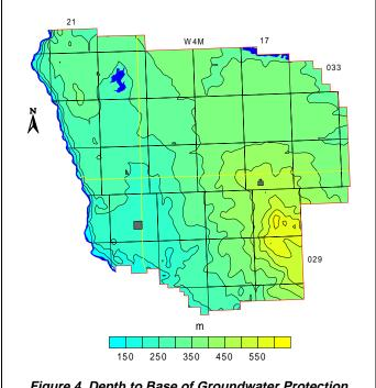
Figure 4. Depth to Base of Groundwater Protection (after EUB, 1995)
