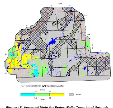
Figure 15. Apparent Yield for Water Wells Completed through Upper Sand and Gravel Aquifer
