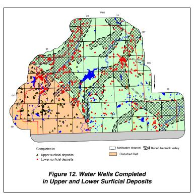
elevation of the completed depth is above the elevation of the bedrock surface determined from the gridded bedrock topographic surface at the same location, then the water well is considered to be completed in an aquifer in the surficial deposits.
