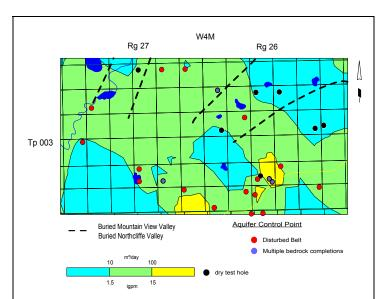
Figure 48. Apparent Yield for Water Wells Completed in Upper Bedrock Aquifer(s) – Area 3
