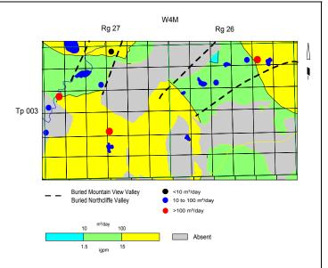
Figure 47. Apparent Yield for Water Wells Completed in Sand and Gravel Aquifer(s) – Area 3
