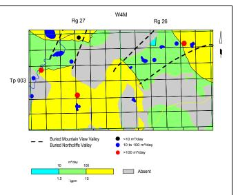
Figure 49. Apparent Yield for Water Wells Completed in Sand and Gravel Aquifer(s) – Area 4
