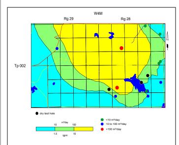
Figure 50. Apparent Yield for Water Wells Completed in Upper Bedrock Aquifer(s) – Area 4
