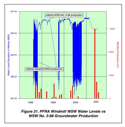
Windmill WSW, as opposed to the groundwater diversion from WSW No. 3-98, as shown on Figure 31.
