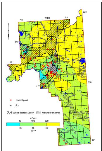
Figure 25. Apparent Yield for Water Wells Completed through the Foremost Aquifer
