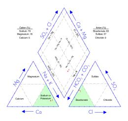
Piper Tri-Linear Diagram
