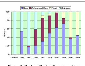
Figure 2. Surface Casing Types used in Drilled Water Wells
