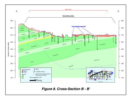
There were 21 bedrock water wells that were completed with a water well screen. Records from 17 of these 21 bedrock water wells indicated the presence of coal in the screened interval.
