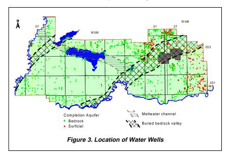
There are 2,024 water well with records sufficient information to identify the aguifer in which the water wells are completed. The water wells that were not drilled deep encounter enough to the bedrock plus water wells that have the bottom of their completion interval above the bedrock surface are water wells completed in surficial aquifers. The number of water wells completed in aquifers in the surficial deposits is 20%, a total of 407 water wells. Ninety-five percent of the surficial water
