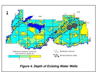
difference between the maximum and minimum depth is more than 30 metres. In the vicinity of linear bedrock lows, the greatest differences between minimum and maximum depth occur. Generally this occurs because aquifers are developed in both the surficial deposits and the bedrock deposits.
