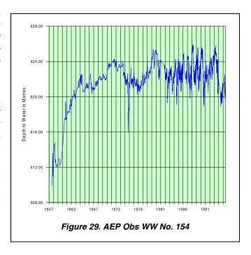
1961, and has continued to be mainly between 620 and 625 metres AMSL. Since April 1993, Husky has been licensed to divert from two water source wells completed in the Lower Sand and Gravel Aquifer: 50.7 m³/day from a water source well in 11-01-050-01 W4M and 169 m³/day from a water source well in 12-01-050-01 W4M. There has been no apparent decline in the Lower Sand and Gravel Aquifer at the site of AEP Obs WW No. 154.
