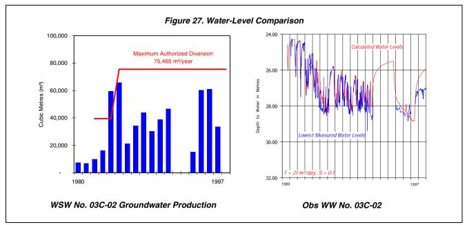
From 1982 to 1991, Dome Petroleum Limited (Dome) diverted 734,461 cubic metres mainly from one water source well completed in the Lower Sand and Gravel Aquifer associated with the Buried Vermilion Valley in 16-10-052-04 W4M. The diverted groundwater had no adverse effect on the quantity of the groundwater available for the Lower Sand and Gravel Aquifer at the site of the Dome Auxiliary Water Well as shown in the adjacent figure (HCL, June 1992).
