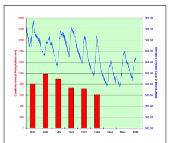
Figure 26. Annual Precipitation vs Water Levels in AEP Obs WW No. 237
