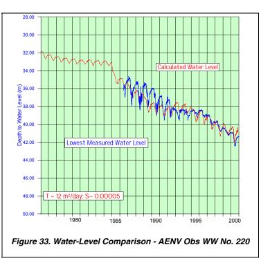
Despite the limited data available, there is a reasonable degree of comparison between the calculated and measured water levels in AENV Obs WW No. 220.
