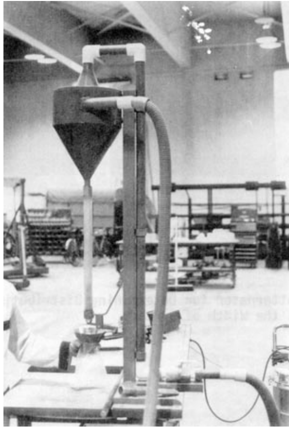
FIGURE 3. Vacuum Cleaner-Cyclone Collection Apparatus.
