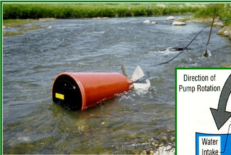
Sling Pump in Operation
