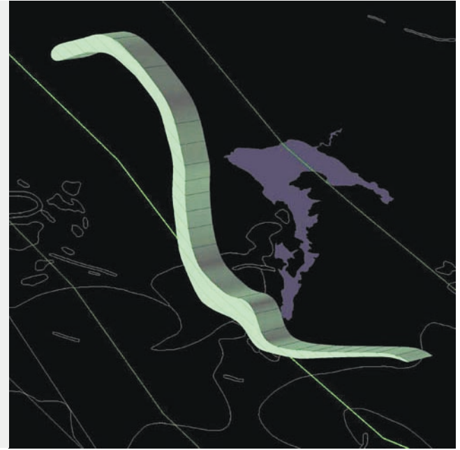
Figure 5. Perspective view of an interpretation that extends Bravo Lake Formation, mafic volcanic klippen along the section line. Section plane cuts topography along thin green line in north-south direction. Note that thickness estimate of the mafic unit is unconstrained. One kilometre structural-contour interval. Perspective view looking northeast.
