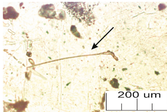
Figure 2. Photomicrograph of hair-like baddeleyite crystal enclosed by sodic plagioclase in coronitic metadiabase from the sample site near Key Harbour.
