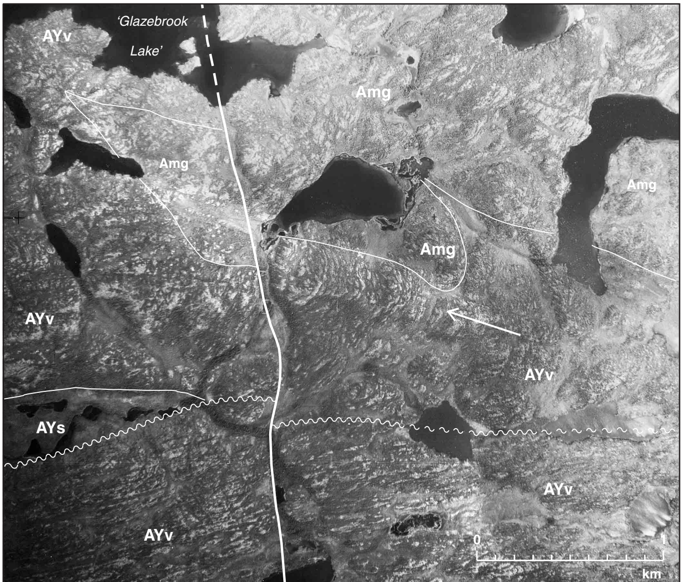
Figure 94. Airphoto of part of the intermediate to felsic dome southwest of 'Glazebrook Lake' showing probable smaller order fold closures within the volcanic dome (arrow). Fine white lines indicate contacts between mainly felsic metavolcanic rocks (AYv) and/or metasedimentary rocks (AYs) and/or metagabbro (Amg). The heavy white line represents a fault while the wiggly line represents a shear zone. Modified from part of NAPL A8749-15
