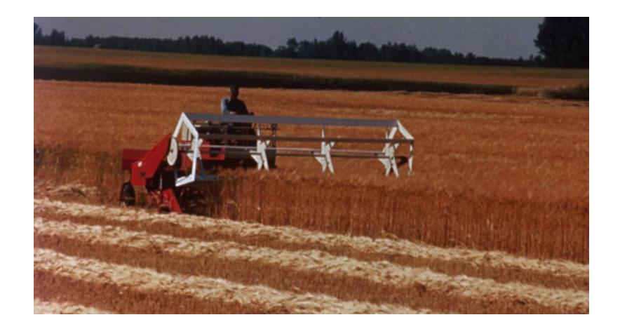
Swathers are used to cut the grain and lay it in rows with the kernels on top to dry.
