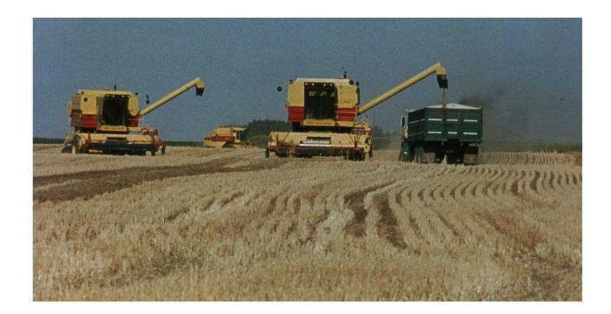
Combines collets the swaths and separate the grain from the straw. The straw is left on the filed and the grain is collected in a hopper, then transferred to trucks.
