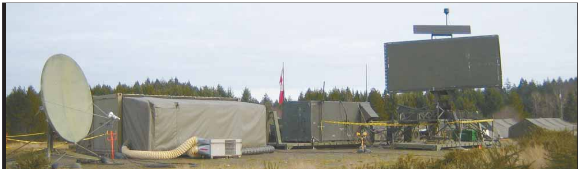
SatCom antenna, MECC shelter (CP and Link Ops), Radar shelter (radar equipment and GCI scopes), TPS-70 radar antenna, 42 Rdr Sqn deployed to Vancouver Island as proof of concept for Vancouver 2010 Olympic surveillance coverage.
