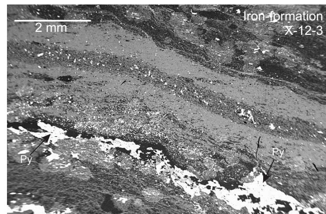
Figure 6. Scanning electron microscopy images displaying sulphide-rich bands (Connell et al., 1999) in an iron-formation sample from Bathurst (New Brunswick), which coincide with the very low electrical resistivity ( \rho_r ) direction of the sample. In this case, the sulphide grains are deformed and show good grain-to-grain connectivity, resulting in low \rho_r values (<10 \Omega\cdot\text{m} ); Py=pyrite.
