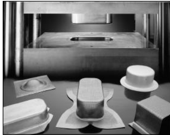
75 tonne press and samples of lightweight formed parts
