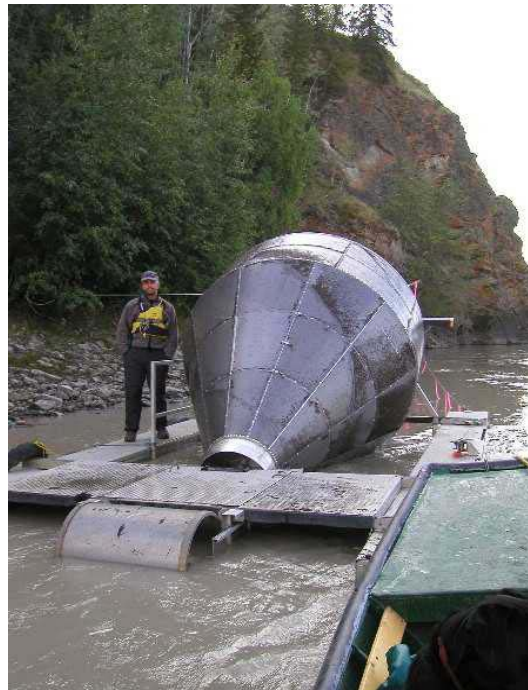
Figure 5. Photograph of the rotary screw trap on site in the Yukon River near Dawson City (courtesy Jim Duncan, Yukon Salmon Commission).
