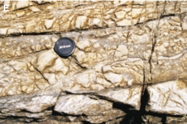
Figure 3. D) Close-up of fault gouge of the St. Lawrence Fault at Sault-au-Cochon. Note the faintly developed fault fabric. E) Fault breccia of the Cap-Tourmente Fault. F) Fault breccia with a composite matrix of crush breccia and pseudotachylyte (dark-coloured material) at Cap-Tourmente.
