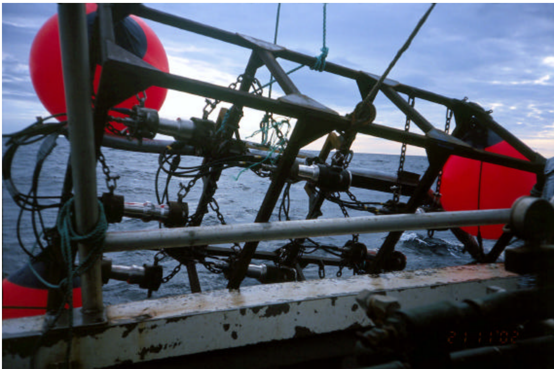
Figure 3. 200-in 3 seven-air gun array in frame.
