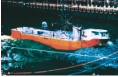
The Terra Nova oil production vessel undergoes seakeeping experiments in IMD's Offshore Engineering Basin.
