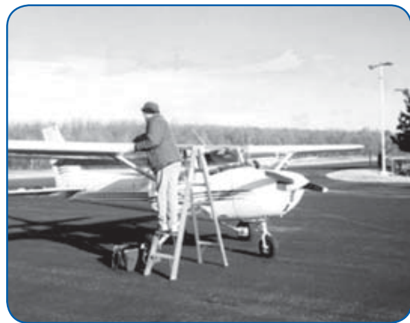
Pilot removing frost manually on small aircraft. Photo: www.Cessna150-152.com .
