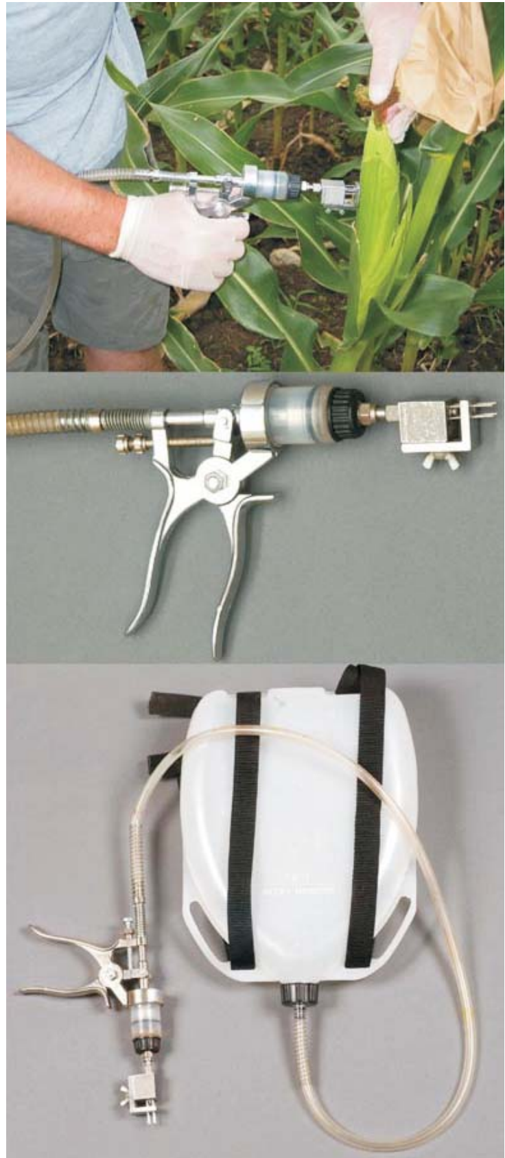
Figure 2. Kernel inoculator used for gibberella and fusarium ear rot inoculations. A graduated, 10 ml, self-refilling, automatic vaccinator is attached to a 2.5 L backpack containing the fungal spore suspension. Two ml of inoculum is injected via four needles into the kernels 10-15 days after silk emergence. The four needles have sealed ends and openings on the underside near the tip to allow puncture and injection without plugging the needle with husk and kernel tissue.
