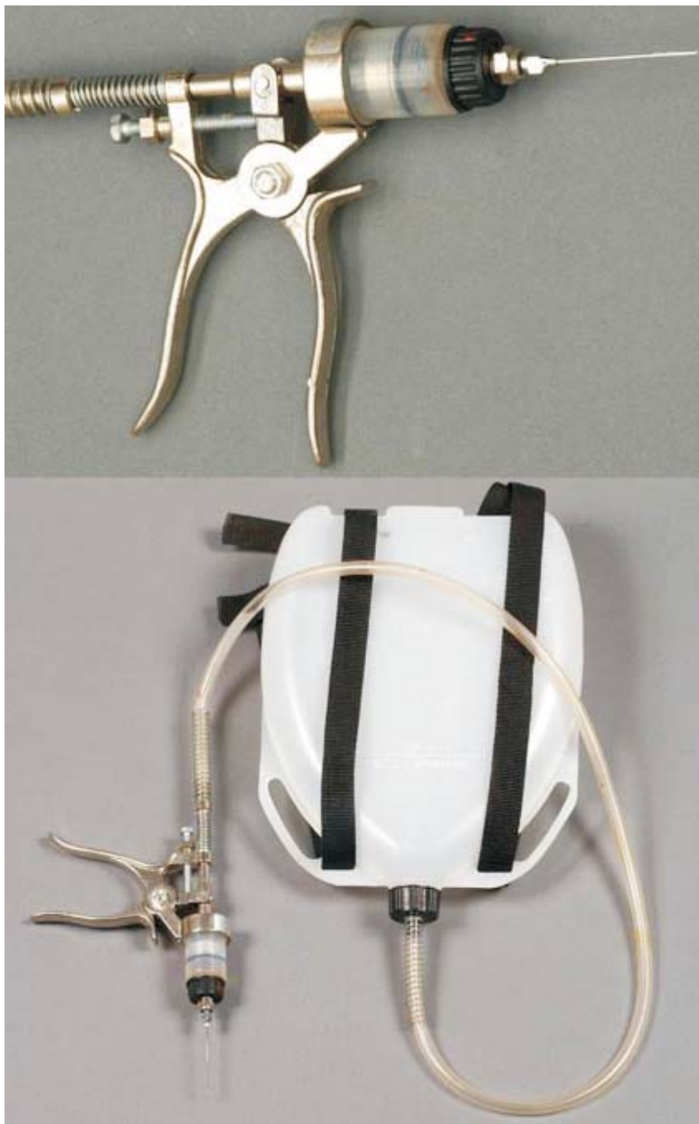
Figure 1. Silk channel inoculator used for gibberella and fusarium ear rot and common smut inoculations. A graduated, 10 ml, self-refilling, automatic vaccinator is attached to a 2.5 L backpack containing the fungal spore suspension. Two ml of inoculum is injected into the silk channel 4-7 days after silk emergence.
