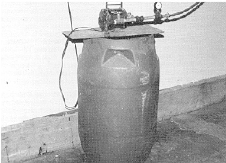
**Fig. 34 Pump and tank used for injecting medicated solution into the drinking water system**
