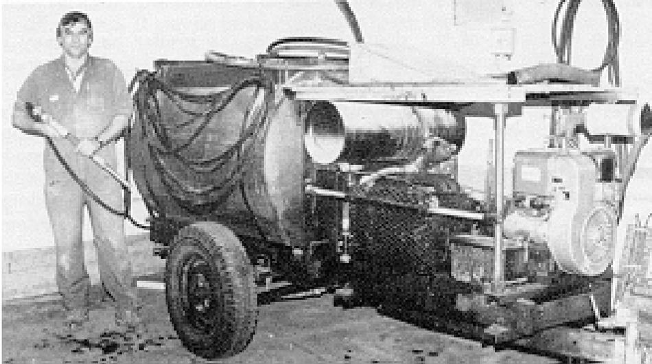
**Fig. 36** A high-pressure sprayer used for washing and disinfecting broiler buildings.
