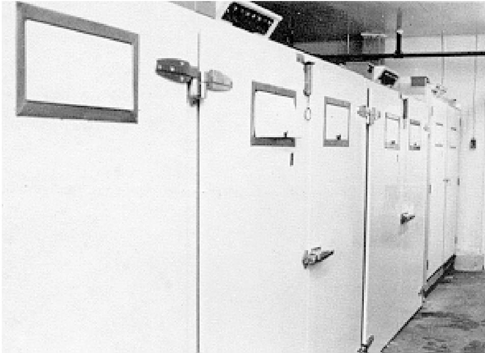
**Fig. 5 Incubators used for the production of broiler chicks.**
