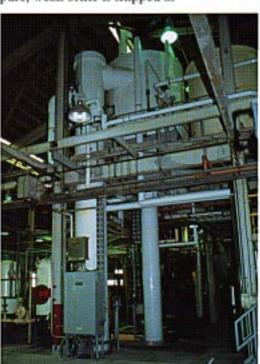
raw material to the sodium chlorate plant. By using this already treated brine, the chlorate plant can avoid having to run a costly treatment system. This dilute brine is concentrated by a double-effect evaporation system. Then, so as to get rid of sodium sulfate still present, a volume of brine which corresponds to 22.7 tonne/d of salt had to be discharged to the sewers.
