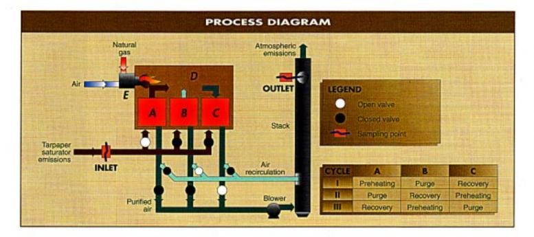
Regenerative incineration can treat emissions containing organic vapour loads varying from 0 to 5000 mg per Nm3. The operation adjusts automatically to variations in emission concentration and flow. For the destruction of organochlorines, combustion temperatures can reach up to 1000°C and more, if required.
