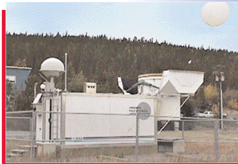
The automated radiosonde launcher at Whitehorse Upper Air Station, Yukon Territory.
