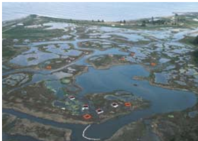
Site of an oil spill bioremediation field experiment in Pepteswick Inlet. The red rectangles are the location of oiled and control plots. Booms to prevent the escape of oil are also visible.
