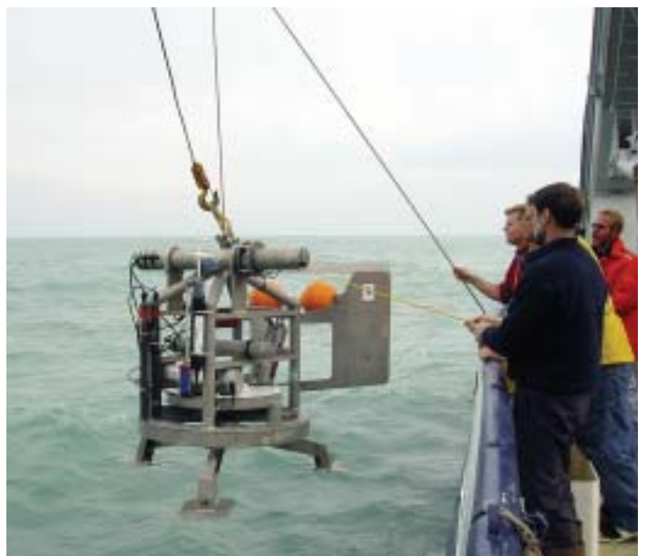
INSSECT being deployed as part of a multidisciplinary study of sediment transport in the western Adriatic.
