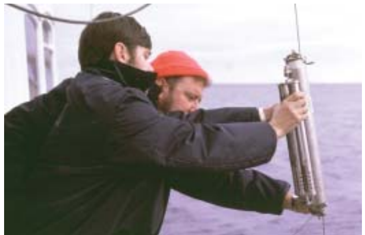
Observing temperature and salinity using a Knudsen bottle and reversing thermometers.
