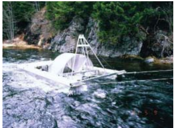
Rotary screw trap used to live-capture Atlantic salmon smolts in the Big Salmon River, N.B. - photo by Ross Jones.
