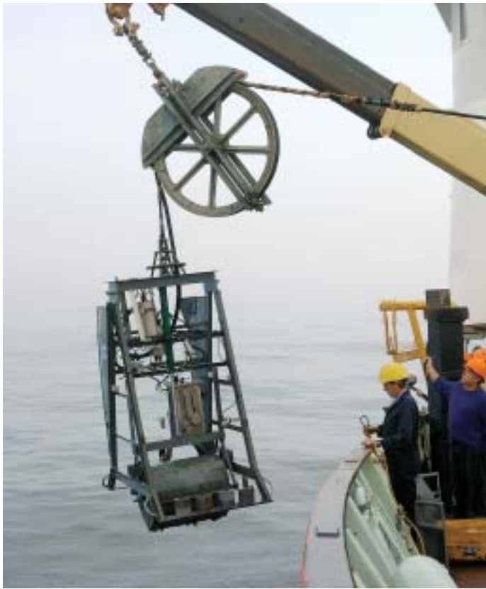
Videograph equipment developed at BIO being deployed on CCGS Hudson, June 2000. Videograph was used in research investigations on the impacts of mobile fishing gear on bottom habitat.
