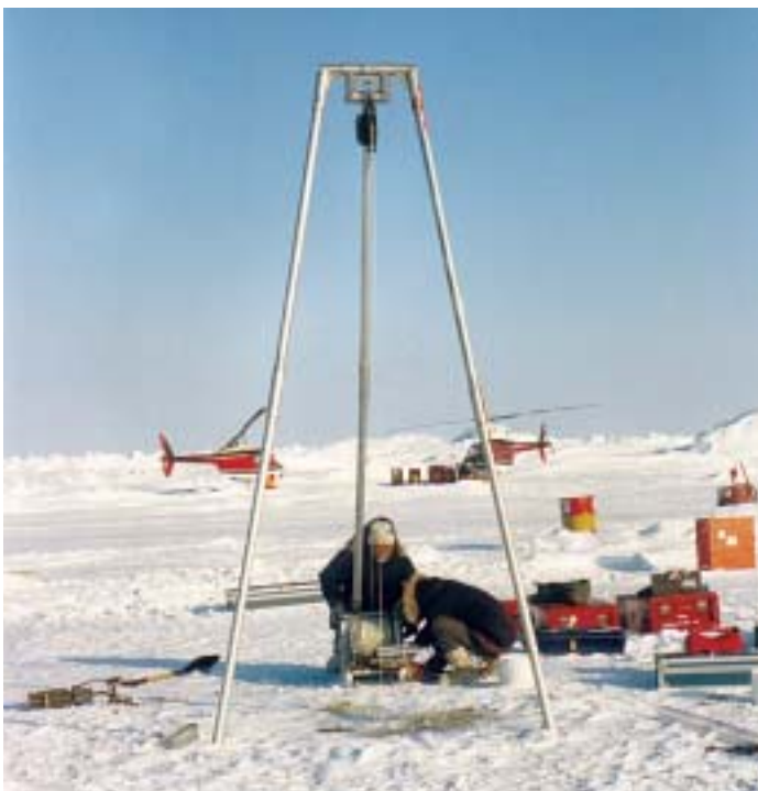
Collection of Vanveen grab samples, mini-gravity cores, and heat flow measurements of the Arctic Ocean seafloor from Hobson's Choice Ice Island (circa 1987) - photo by David Mosher.
