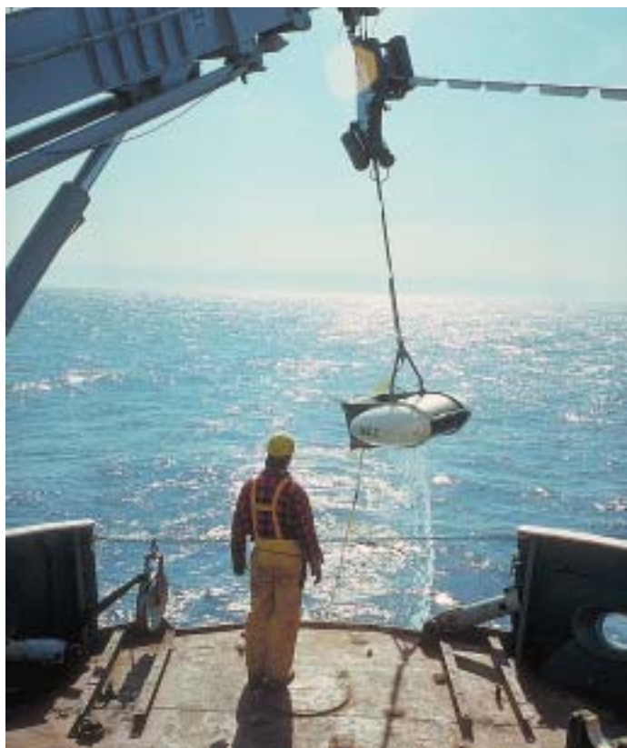
Huntec Deep-Towed Seismic Reflection System (DTS™) was developed in an industry-BIO partnership in the 1970s, and used throughout the world for deep seismic profiling.
