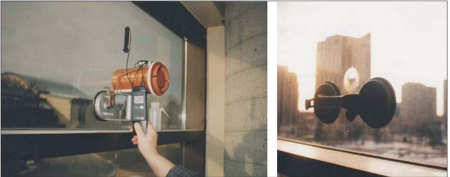
Figure 4: Field dew-point measurement apparatus: (Left) The unit is mounted on an insulating glass unit in contact with the inboard pane of glass. A digital thermometer inserted into the unit measures the temperature of unit in contact with the pane. (Right) The apparatus has been removed (except for the suction cups), revealing a circle of condensation or frost on the cavity-side surface of the pane, directly beneath the chilled contact area of the apparatus.
