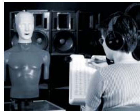
A talking mannequin is used to study speech reception in noisy environments such as ship operations rooms.
