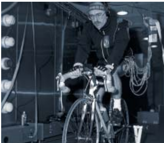
Our climatic and physiological monitoring facilities at DCIEM are used to assess the protective capabilities of technical clothing for the Canadian Forces.
