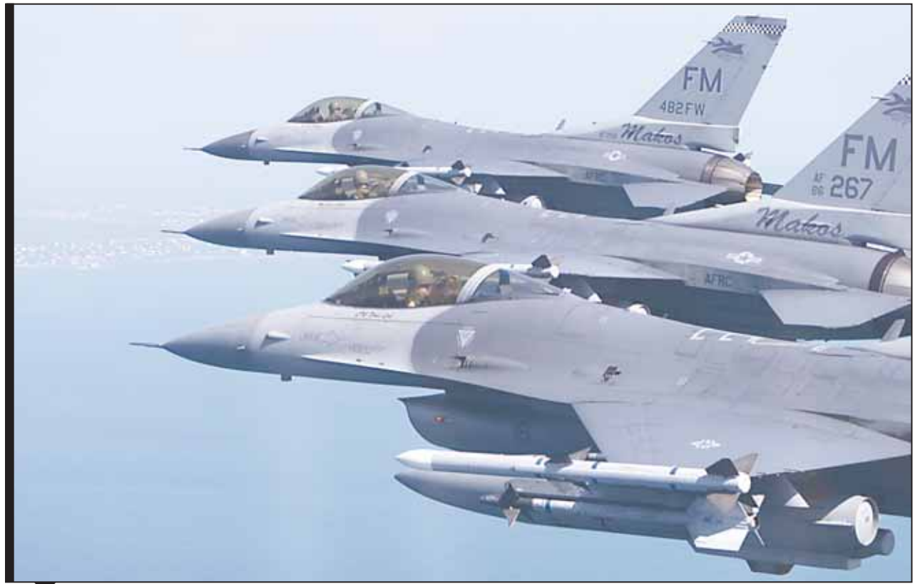
482nd Fighter Wing/93rd Fighter Squadron in a three-ship formation of Lockheed F-16C Fighting Falcons carrying AIM-120 and AIM-9 air-to-air missiles.
