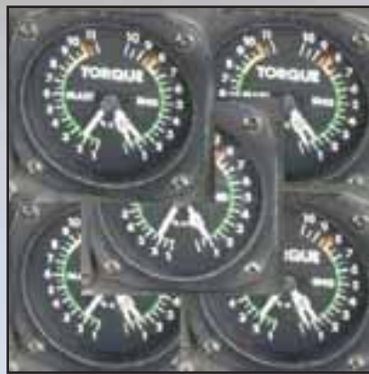
A collage of Griffon torque gauges showing “the split” — not exactly representative of flight conditions but you get the idea.
