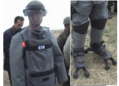
Med-Eng Systems Inc.'s HDE full body protective suit, HDH demining helmet and spiderboots.
