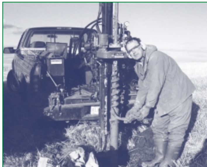
An NWRI technician installs piezometers—instruments used to measure the magnitude or direction of pressure—near Elstow, Saskatchewan, as part of a project to monitor prairie water quality.
