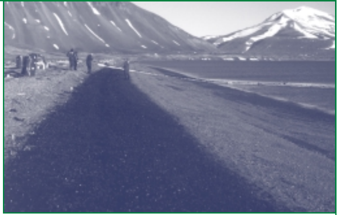
Swath of oil applied to a beach test site in the Svalbard islands, north of Norway.
