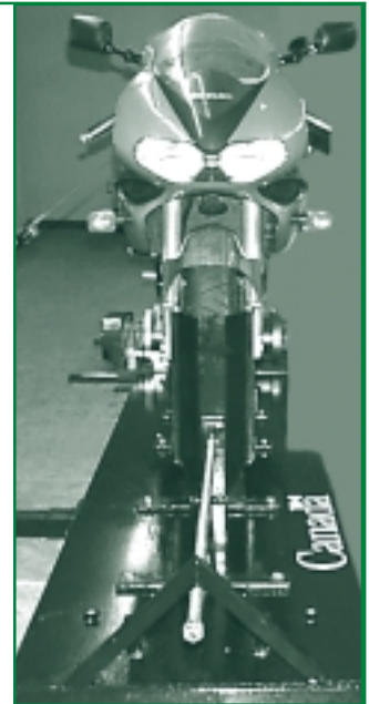
A motorcycle mounted on a dynamometer undergoes emissions testing at the Environmental Technology Centre in Ottawa.
