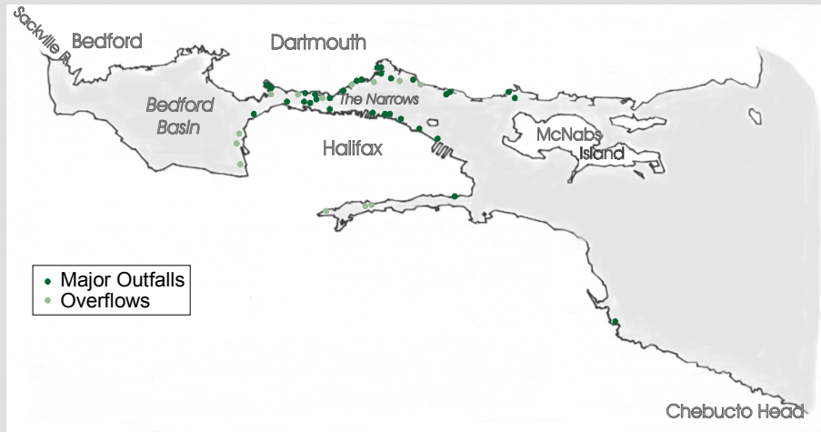
Figure 4.9. Halifax Harbour showing locations of major sewer outfalls and overflows. Adapted from EP-EARP 1993.
