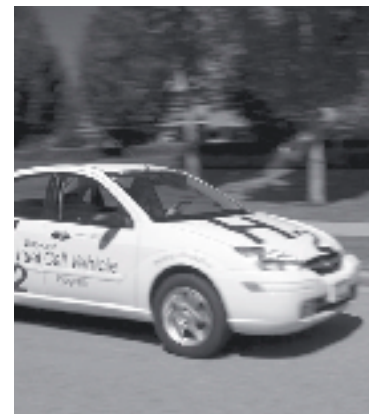
Ford Focus Fuel Cell Vehicle powered by Ballard's mark 902 fuel cell.
