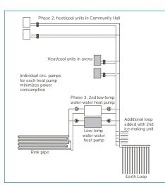
HDPE Pipe laid in ice rink Vertical Earth Loop 48 boreholes, 38 m depth Ice Rink Ice Rink Ice Rink Heat/cool Wunits for rink
