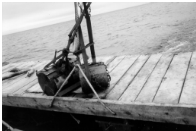
Van-Veen grabs used to collect sediment for toxicity and chemical testing. Source: P. Topping
