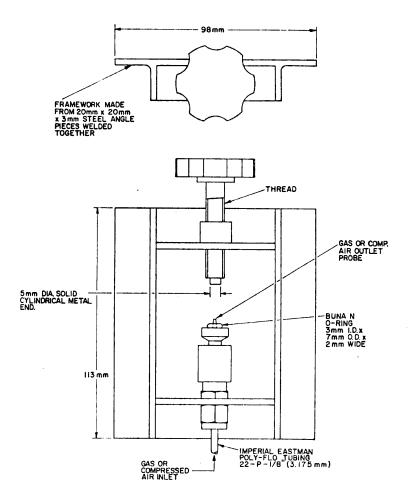
Figure 1: Pressure Test Device
