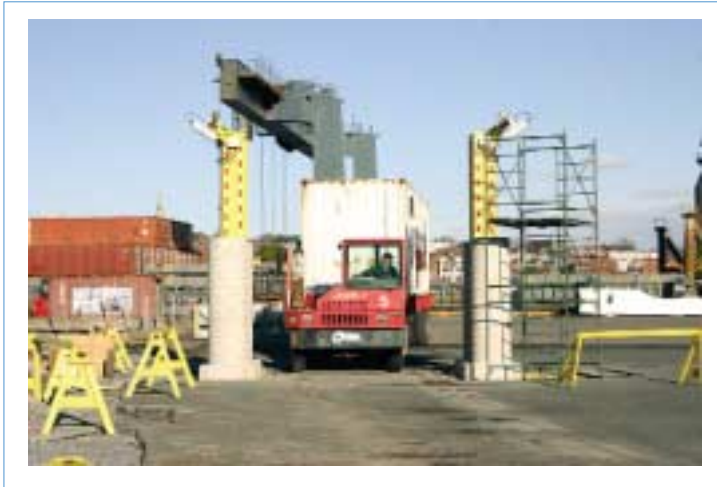
A cargo container is transported by truck through a portal monitor.
