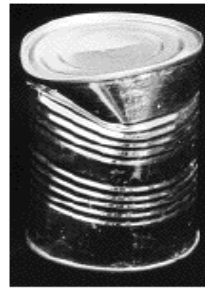
Sharp dent or dent on seam
