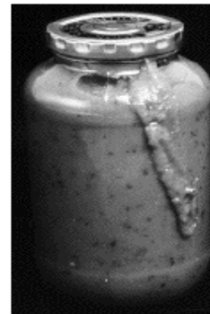
Leaking, crack or chips, or product discolored.
