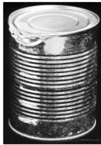
Dented at junction of side and end
