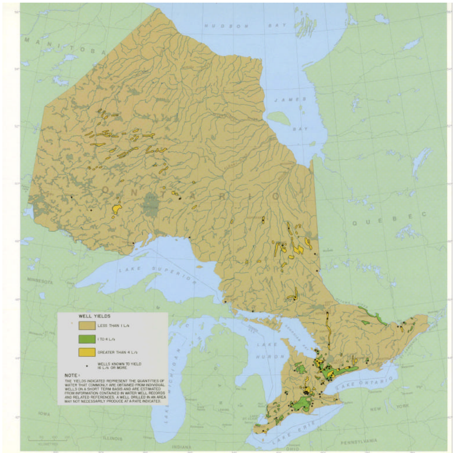
Figure 2.4: Groundwater Yields from Overburden in Ontario (from “Water Quantity Resources of Ontario, MNR 1984)
